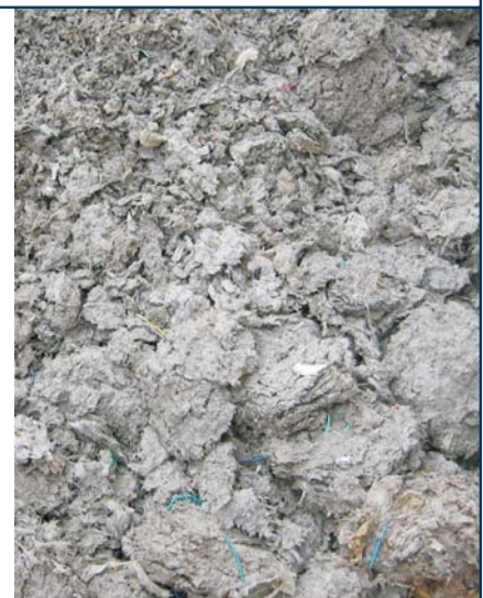
Washed and dewatered screenings
