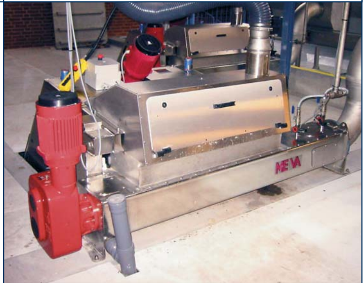
Washing and dewatering
