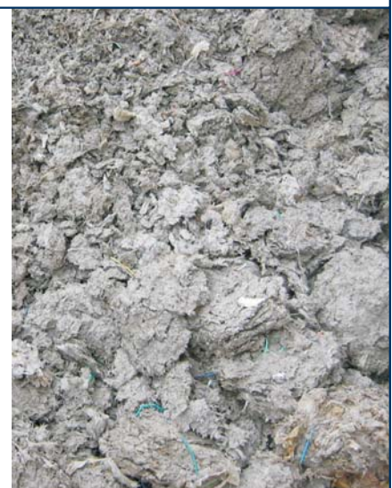
Washed and dewatered screenings
