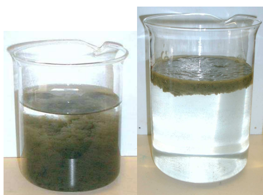
Flotation test to size one flottator
