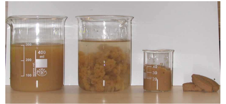
Rough sludge Flocculated sludge Thickened sludge Dewatered sludge
