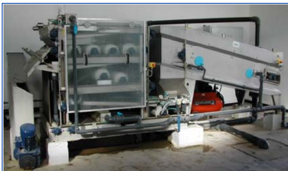
Gravity belt thickener combined with in-line belt filter press
